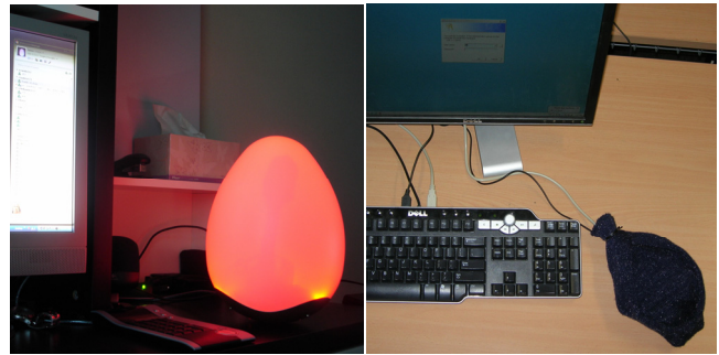
Figure 2. Ambient display artifact examples. Left: an egg shaped USB device that wiggles and moves in reaction to emotions communicated during online chat conversations (Designer: James Kim); Right: a working computer mouse that changes temperature hot/cold depending on the input of textual humans emotions (Designer: Irene Chen).
