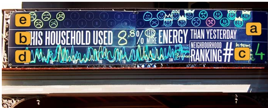
Figure 2. Overview of the graphical depictions on the public feedback display: Marginal Notes (a), Daily Performances (b), Neighborhood Ranking (c), Historical Graph (d), Pictorial Bar (e).
