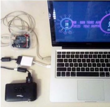
Figure 2. Technical components of the prototype: laptop running the Friends mode visualization, compass module, Arduino microcontroller, and pico projector.
