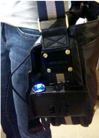
Figure 3. The shoulder bag containing the technical components with the pico projector attached to the side, pointing upwards.
